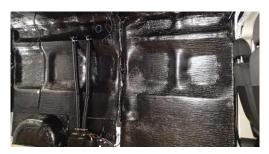
**SOUND DEADENING INSULATION**Reduces sound & insulates to improve climate controls
